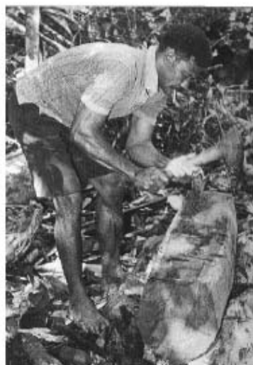
17.1 (Above left) Easi Qalo, master lali -maker of Namuka, starts the initial flattening of the top of the vesi log.
